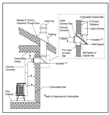
Figure 15A - Exterior Chimney
